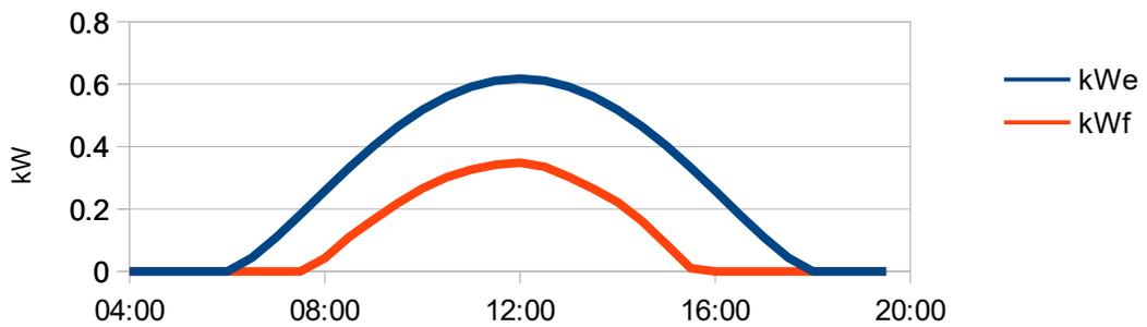
Fig 11: PV generation and feed in profiles
