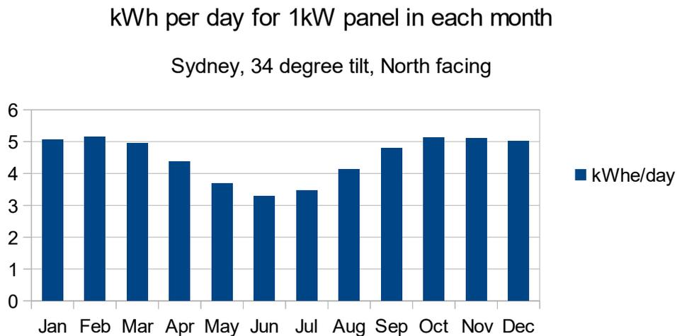
The overall amplitude is adjusted to fit the generally agreed average power over a year in Sydney, namely, 3.9kWh/day for each kWp.
